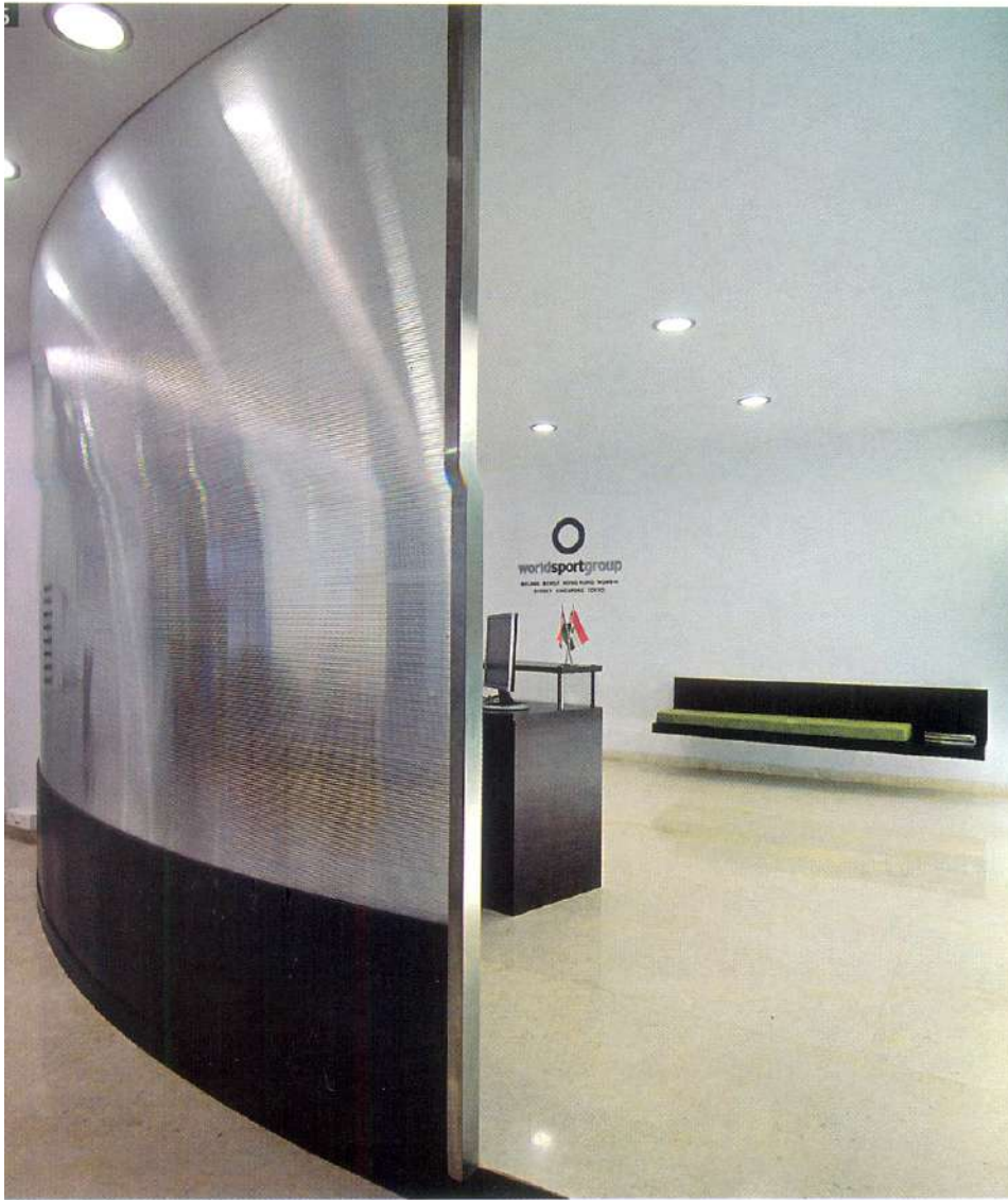
[5] A subtle colour palette in white follows throughout the office. Light materials such as glass and polycarbonate are used to form internal walls. The floor is in a pleasant pink shade of stone called Omani Pink
